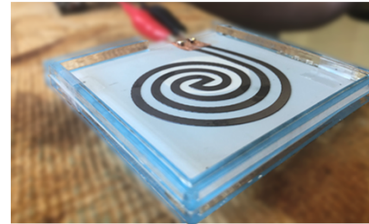
Spray Coated MXene Coil Adhered to Diaphragm
